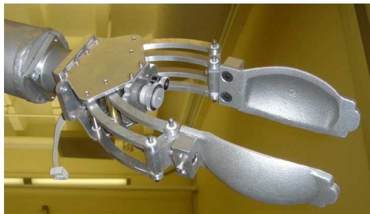
Figure 9.14: The New Gripper and the Actuation Mechanism.
