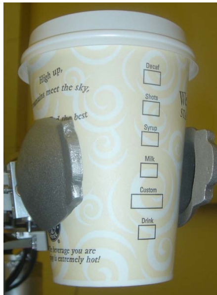
Figure 9.16: The New Gripper When Holding a Tapered Cup.
