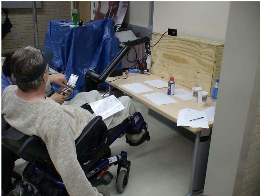
Figure 6.5: Clinical Testing of the Keypad by a Power Wheelchair User.
