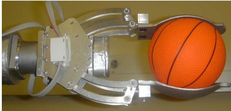
Figure 9.15: The New Gripper When Holding a Spherical Object.
