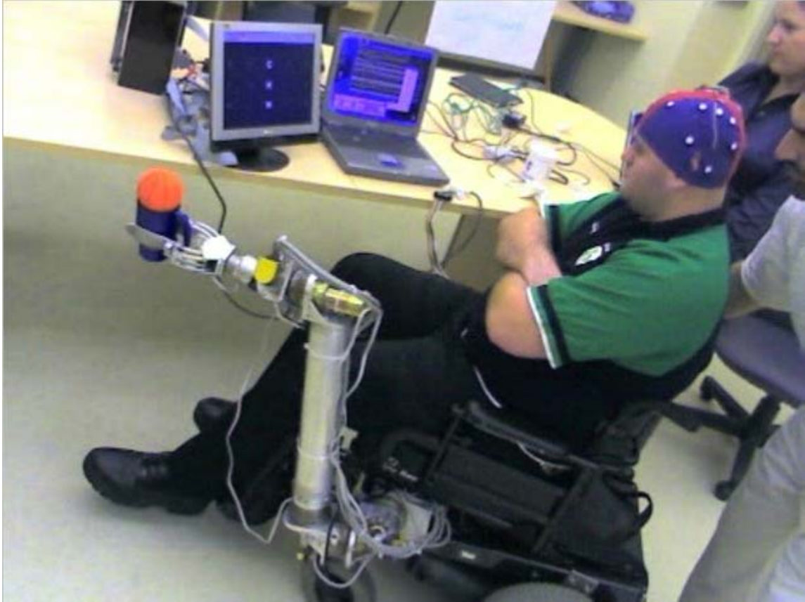
Figure 9.28: A Human Subject Testing of the BCI-2000 Interface with the WMRA System.
