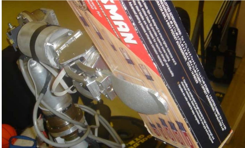
Figure 9.19: The New Gripper When Handling Large and Heavy Objects.
