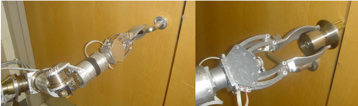
Figure 917: The Gripper When Opening a Door with a Lever Handle (Left) and a Knob Handle (Right).
