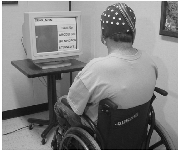
Figure 6.12: The Non-Invasive BCI Device.
