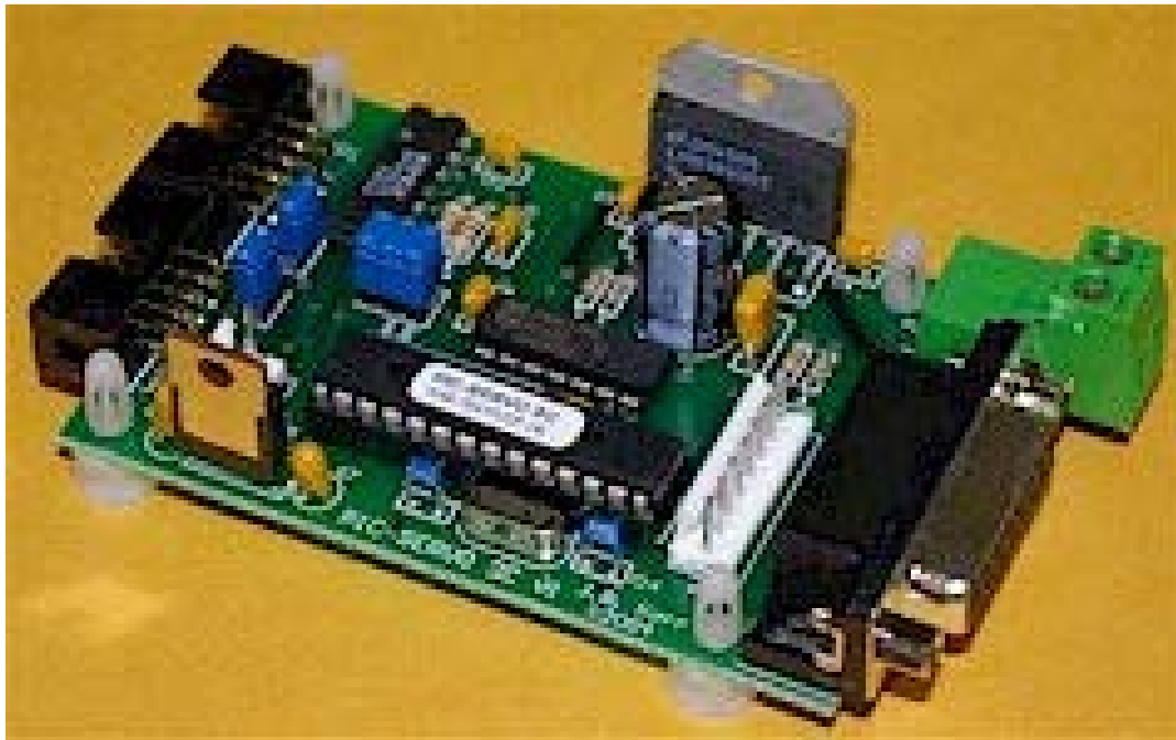
Figure 9.23: JRKERR PIC Servo SC Controller Boards.
